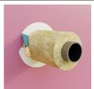
Using a spatula, apply PiroCoat A on the partition in such a way that a ring with a width of min. 50 mm and a thickness of min. 0.6 mm is created
