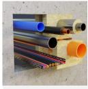
Fill the hole in the wall with mineral wool boards with a minimum density of 150 kg/m³ and a minimum thickness of 50 mm
