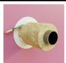
Apply **PiroCoat A** on the pipe cover to form a ring with a width of min. 50 mm and a thickness of min. 0.6 mm
